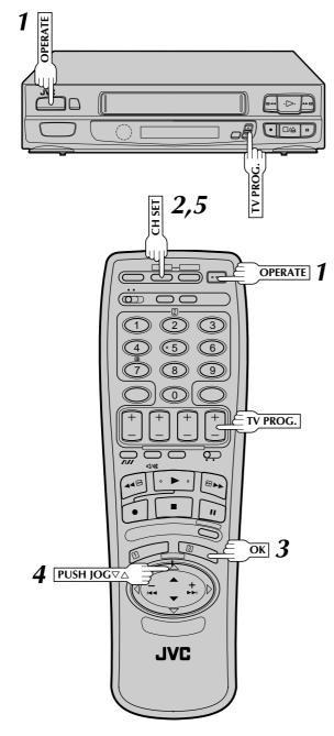
Your recorder needs to memorise all necessary stations in preset positions in order to record TV programmes. ATS+ (Auto Tuning System) automatically assigns all receivable stations in your area to call them up with the **TV PROG.** buttons without going through any vacant channels.
